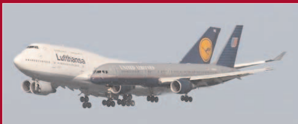
A Lufthansa 747-400 and a United 757-200 are on a simultaneous landing approach on the parallel runways 28L and 28R at SFO. The real runway separation is 225 meters. Due to the telephoto distortion, the Jumbo 747 being three times larger than the 757 and being behind it, gives us this fantastic optical illusion that they are flying inches from each other!!!
